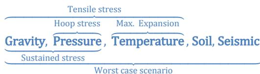
Decisive for the design is the worst case scenario, which consists of sustained stress, hoop stress, maximum expansion and tensile stress as a combination of the previous mentioned stresses, as well as soil and other loads like seismic activity.
